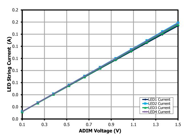
Figure 24 – 4 x 30 V String LED Current vs. ADIM Voltage at 230 VAC.
