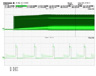
Figure 44 – SR FET Voltage Waveforms. 265 VAC Input, Full Load, (42.1 V<sub>MAX</sub>).
