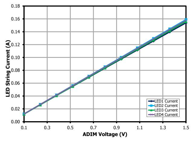
Figure 33 – 4 x 40 V String LED Current vs. ADIM Voltage at 230 VAC.
