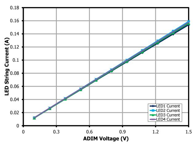
Figure 22 – 4 x 30 V String LED Current vs. ADIM Voltage at 115 VAC.
