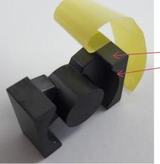
Tape edge to line up with inner edge of core bottom.
