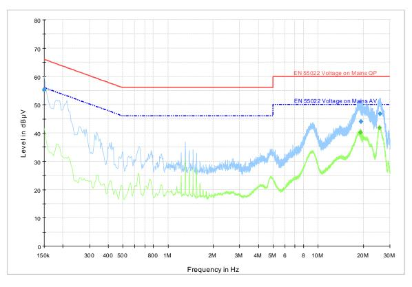
**Figure 72** – Conducted Emissions: 115VAC Input. Output GND connected to ground plane.
