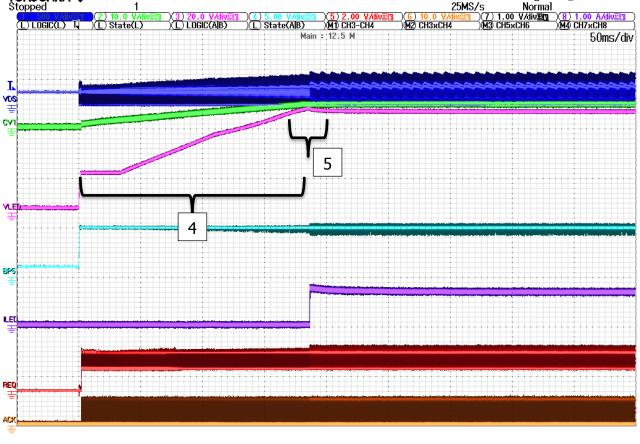
Max(C1) 341 V Max(C3) 43.15 V Figure 7 – Complete Start-Up Cycle Over Approximately 230 ms.
