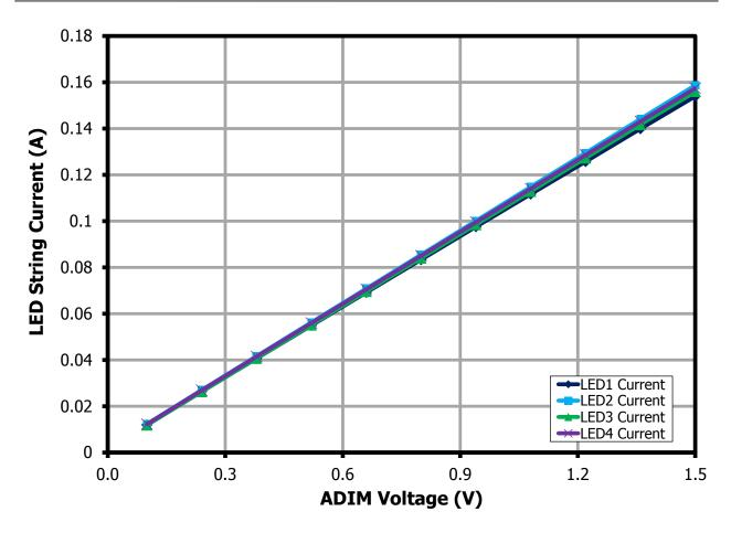
Figure 20 – 4 x 30 V String LED Current vs. ADIM Voltage at 90 VAC.
