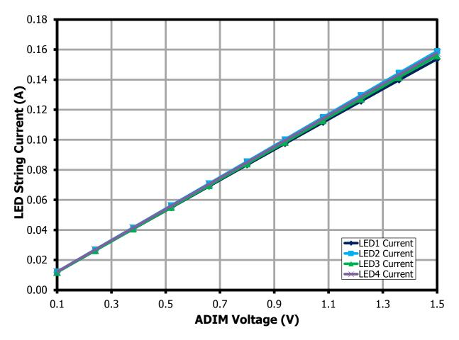
**Figure 31** – 4 x 40 V String LED Current vs. ADIM Voltage at 115 VAC.
