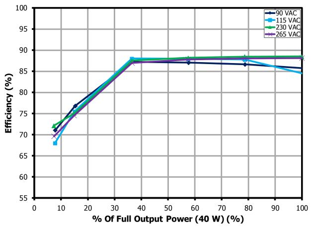
Figure 15 – Efficiency vs Output Power with 40 V LED Strings.
