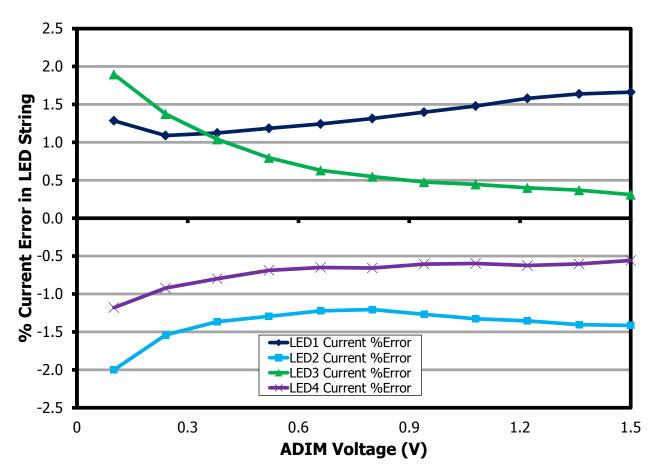
Figure 21 – LED String Current Matching Error for 30 V LED Strings at 90 VAC.
