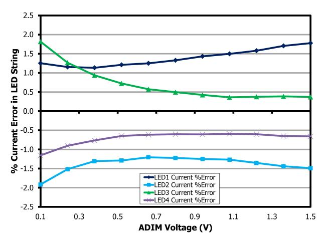
Figure 27 – LED String Current Matching Error for 30 V LED Strings at 265 VAC.
