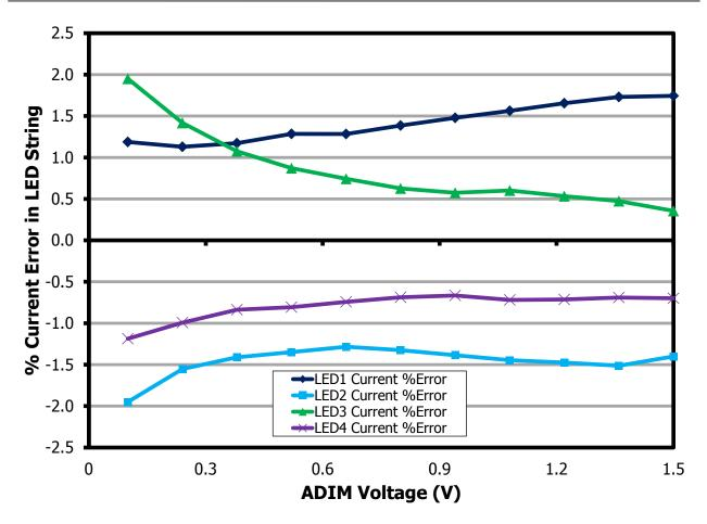
Figure 30 – LED String Current Matching Error for 40 V LED Strings at 90 VAC.
