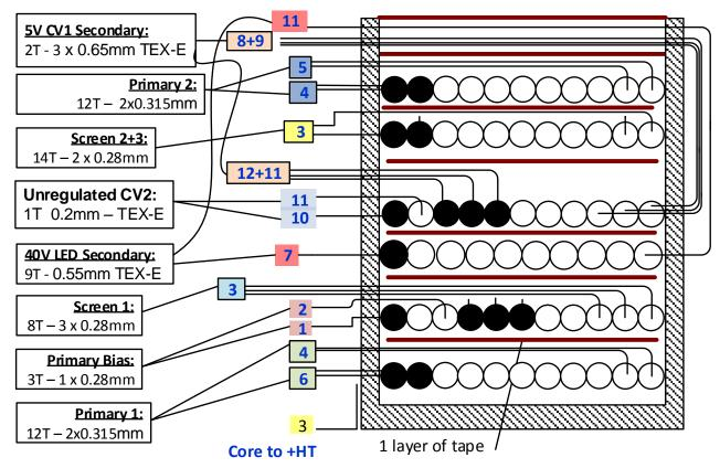
Figure 12 – Transformer Winding Stack
