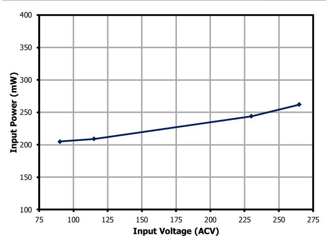
**Figure 37** – Input Power vs. Input Voltage, Room Temperature.
