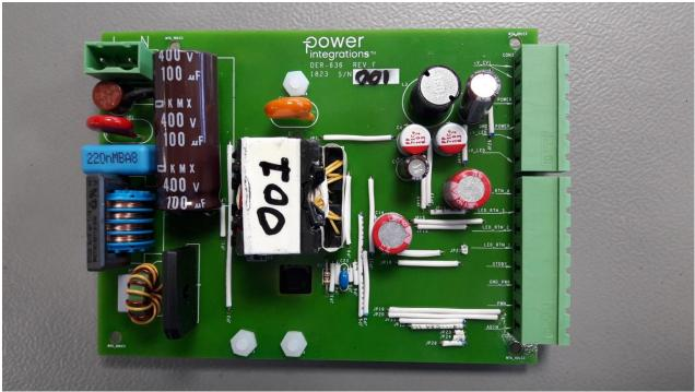
Figure 2 – PCB Assembly – Top View.
