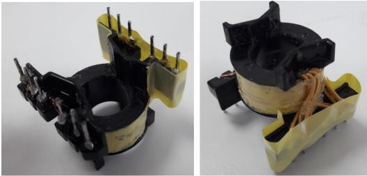
Cut a piece of 6cm x 12mm tape Item [10] and apply it side surface of the core half • way along as shown. The edge of the tape is to be level with the inside edge of the bottom of the core as shown.
