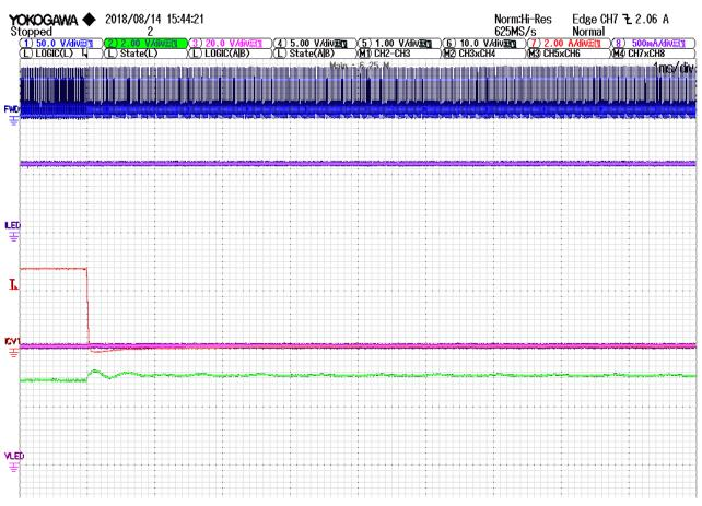
Figure 41 – 5 V Output Load Transient 3A to 50 mA with 625 mA Total LED Current.
