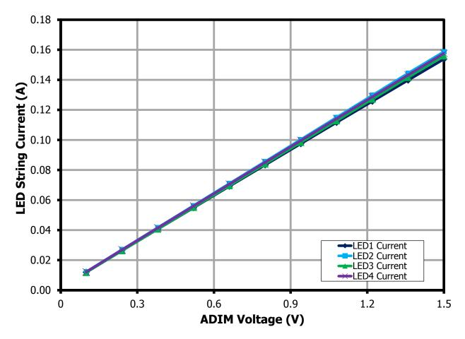
**Figure 29** – 4 x 40 V String LED Current vs. ADIM Voltage at 90 VAC.
