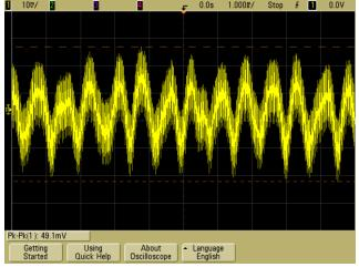
Figure 70 –  $V_{IN}$  = 230 VAC.  $V_{RIPPLE_CV1}$  = 49.1 mV<sub>PK-PK</sub>. CH1: V\_CV1, 10 mV / div. (ac) , 1 ms / div.
