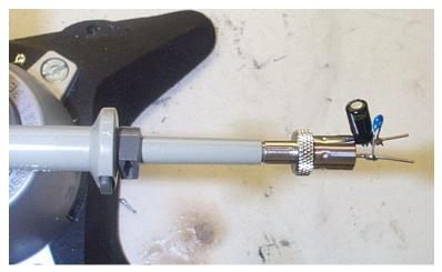
**Figure 64** – Oscillocope Probe with modified BNC Adapter. Probe Master (<u>www.probemaster.com</u>) 4987A BNC Adapter. (Modified by adding two parallel decoupling capacitors and wires for ripple measurement)
