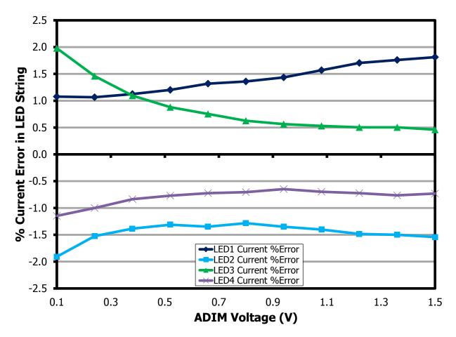
Figure 34 – LED String Current Matching Error for 40 V LED Strings at 230 VAC.
