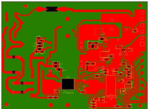
**Figure 10** – Printed Circuit Layout, Bottom.
