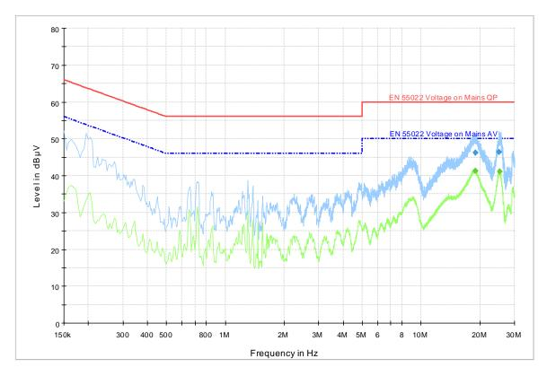
**Figure 73** – Conducted Emissions: 230VAC Input. Output GND connected to ground plane.
