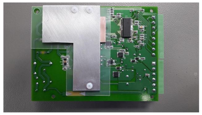
Figure 3 – PCB Assembly – Bottom View, with Heat Sink.
