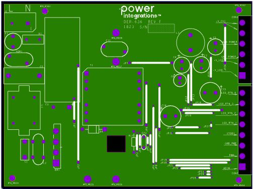
Figure 9 – Printed Circuit Layout, Top.
