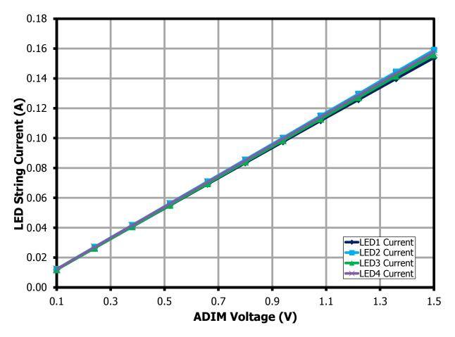
**Figure 35** – 4 x 40 V String LED Current vs. ADIM Voltage at 265 VAC.
