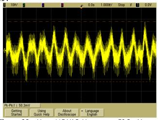
Figure 66 –  $V_{IN}$  = 115 VAC.  $V_{RIPPLE_CV1}$  = 50.3 m $V_{PK-PK}$ . CH1: V\_CV1, 10 mV / div. (ac) , 1 ms / div.
