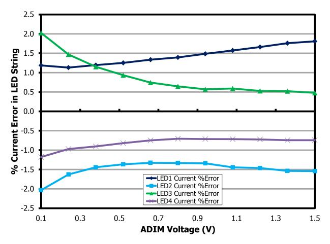
Figure 36 – LED String Current Matching Error for 40 V LED Strings at 265 VAC.
