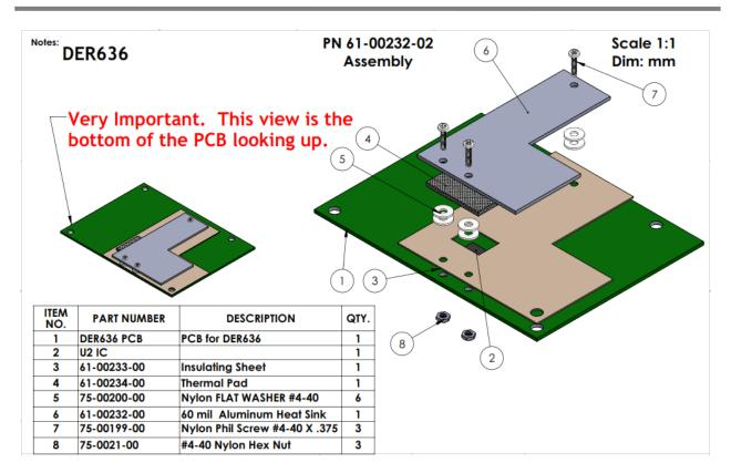
Figure 78 – Heat Sink Assembly Drawing.
