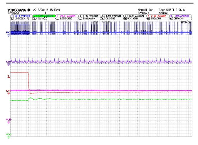
Figure 39 – 5 V Output Load Transient 3A to 50 mA with 63 mA Total LED Current.
