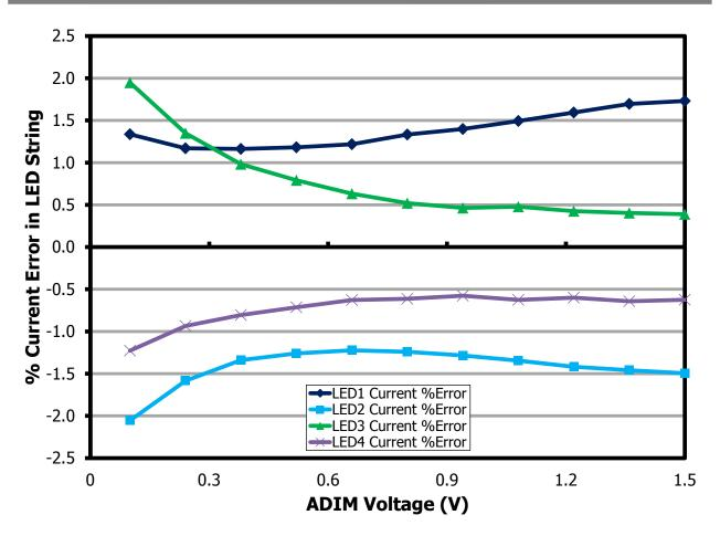
Figure 23 – LED String Current Matching Error for 30 V LED Strings at 115 VAC.
