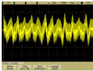
Figure 68 –  $V_{IN}$  = 265 VAC.  $V_{RIPPLE_CV1}$  = 51.9 mV<sub>PK-PK</sub>. CH1: V\_CV1, 10 mV / div. (ac) , 1 ms / div.
