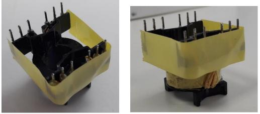
• With the back edge of a scalpel, push the tape to stick to the inner surfaces as shown, ensure the tape goes right up to the corners.
