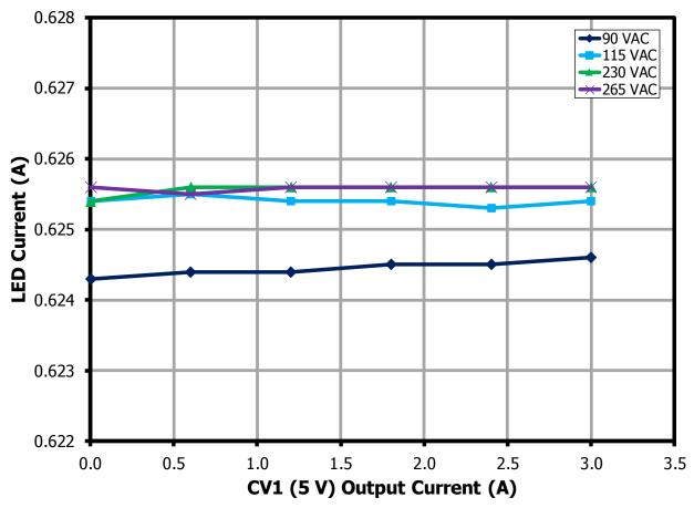
11.3 LED Current Cross Regulation with CV1 Load and VAC
