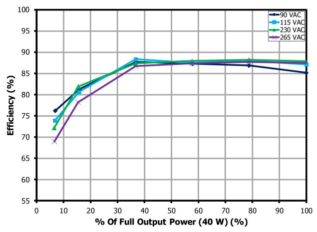
Figure 14 – Efficiency vs Output Power with 30 V LED Strings
