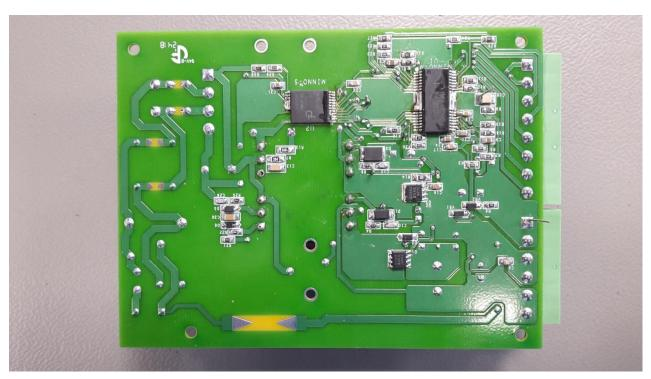
**Figure 4 –** PCB Assembly – Bottom View, without Heat Sink.
