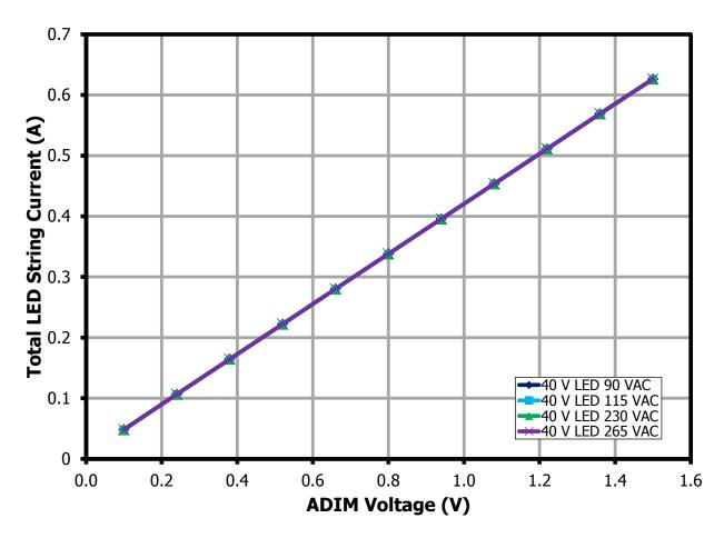
Figure 28 – Total LED Current vs. ADIM Input Voltage for 40 V LED Strings.
