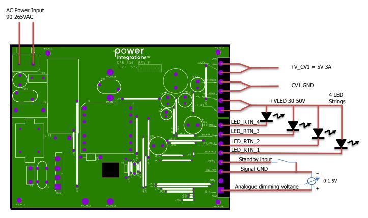
Figure 8 – DER-636 Connection Diagram.
