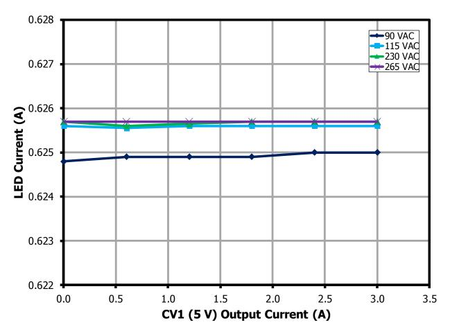
Figure 18 – Effect of CV1 Load and VAC Input on LED Current, 40 V LED Strings.
