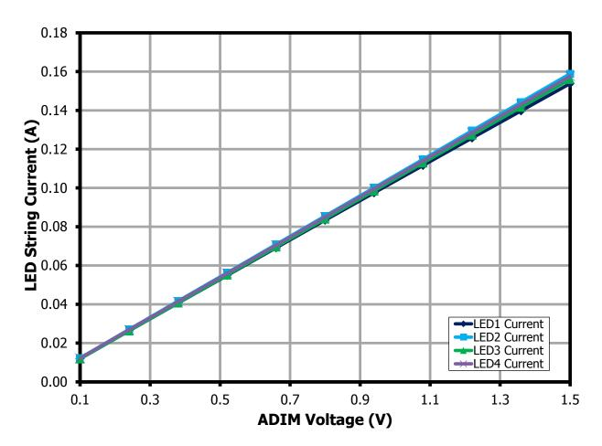
Figure 26 – 4 x 30 V String LED Current vs. ADIM Voltage at 265 VAC.
