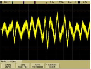
Figure 69 –  $V_{IN}$  = 115 VAC.  $V_{RIPPLE_{CV1}}$  = 44.0 mV<sub>PK-PK</sub>. CH1: V\_CV1, 8 mV / div. (ac) , 1 ms / div.
