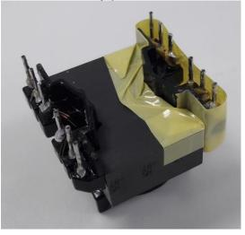
Insert top core half and secure with 2 layers of tightly wound 6 mm tape Item
