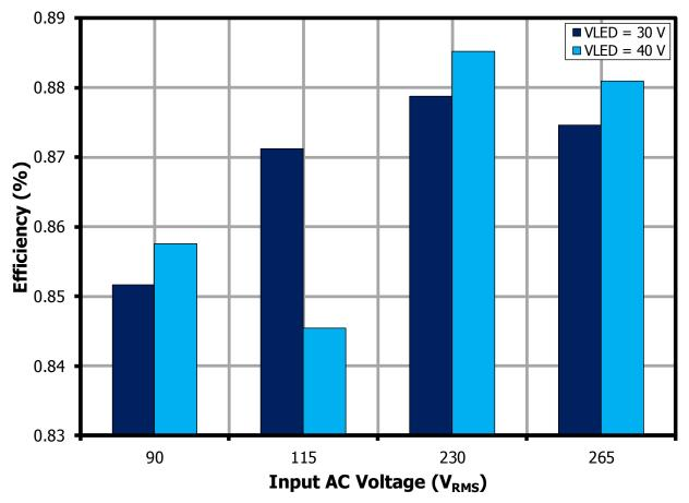
Figure 13 – Full Load (40 W) Efficiency vs. Line; Room Temperature
