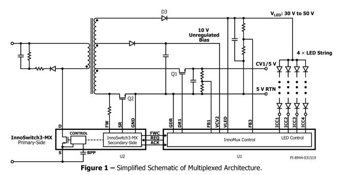
This novel architecture is implemented using two controller ICs, the InnoSwitch3-MX IC for primary switching plus SR FET control, and InnoMux IC for output voltage and current control. Selection MOSFET Q1 and D3 are used to direct the energy packet to either the CV or LED output respectively.
