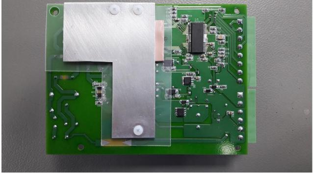
Figure 74 – Populated Circuit Board Photograph, with Heat Sink.
