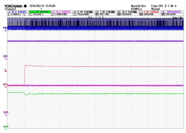
Figure 40 – 5 V Output Load Transient 50 mA to 3 A with 625 mA Total LED Current.
