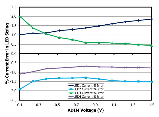
Figure 32 – LED String Current Matching Error for 40 V LED Strings at 115 VAC.
