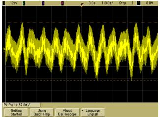
Figure 67 –  $V_{IN}$  = 230 VAC.  $V_{RIPPLE_{CV1}}$  = 57.8 mV<sub>PK-PK</sub>. CH1: V\_CV1, 12 mV / div. (ac) , 1 ms / div.
