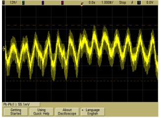
$\begin{array}{l} \mbox{Figure 65} - V_{IN} = 90 \mbox{ VAC. } V_{RIPPLE\_CV1} = 55.1 \mbox{ mV}_{PK\text{-}PK}. \\ \mbox{ CH1: } V\_CV1, \ 12 \mbox{ mV} \ / \mbox{ div. } (ac) \ , \ 1 \mbox{ ms} \ / \mbox{ div.} \end{array}$
