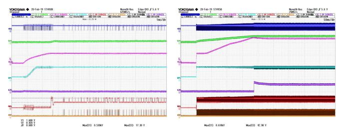
Figure 55 – Input 265 VAC. Initial Start-up 1st 10 ms. Output CV1 = 5 V @ 15 W, LED = 40 V @ 625 mA.
