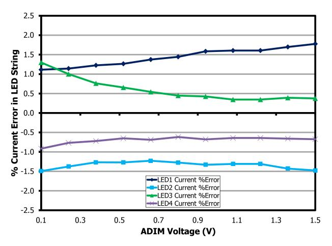
Figure 25 – LED String Current Matching Error for 30 V LED Strings at 230 VAC.
