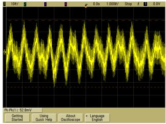
Figure 71 –  $V_{IN}$  = 265 VAC.  $V_{RIPPLE_{CV1}}$  = 52.8 mV<sub>PK-PK</sub>. CH1: V\_CV1,10 mV / div. (ac) , 1 ms / div.
