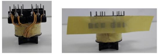
• Fold both sides over to stick to the sides of the secondary pin support moldings.
