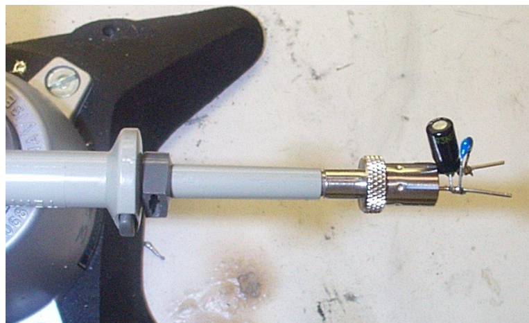
Figure 93 – Oscilloscope Probe with Probe Master ( www.probemaster.com ) 4987A BNC Adapter. (Modified with wires for ripple measurement, and two parallel decoupling capacitors added)
