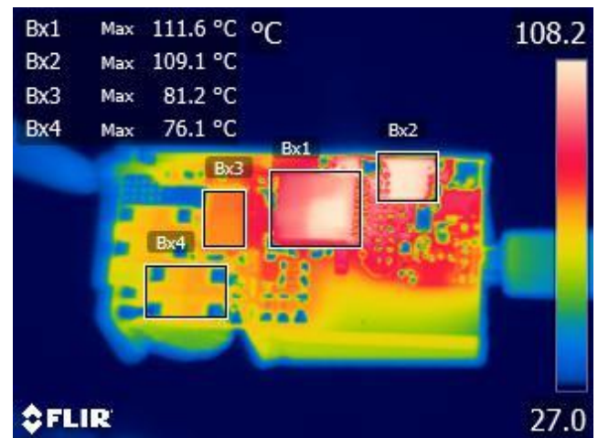
Figure 45 – Bottom Thermal Image.
