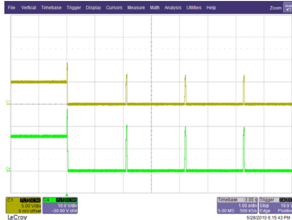
Figure 24 – Output Overvoltage Protection, 90 VAC. Top: 5 V Output Voltage, 5 V / div. Bottom: 16 V Output Voltage, 10 V / div., 1 ms / div.
