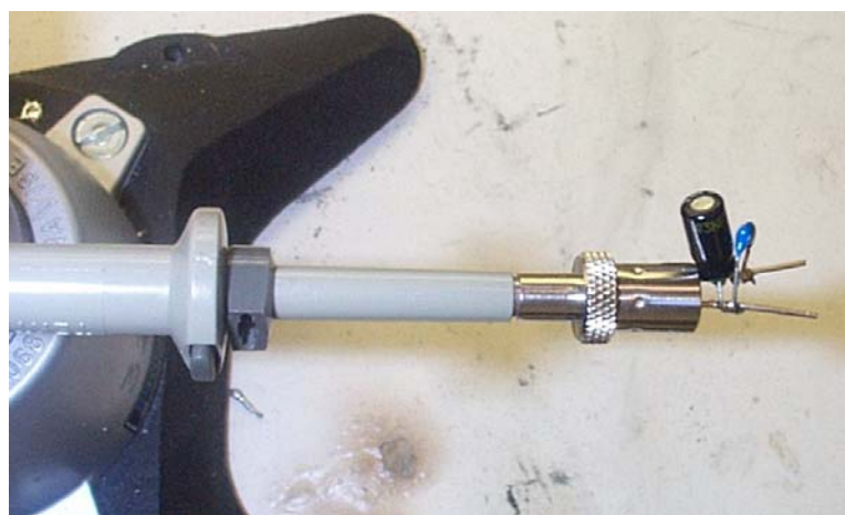
Figure 26 – Oscilloscope Probe with Probe Master ( www.probemaster.com ) 4987A BNC Adapter. (Modified with wires for ripple measurement, and two parallel decoupling capacitors added)
