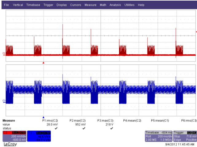
Figure 47 – 90 VAC, 60 Hz Output Short Condition. Upper: I_{DRAIN} , 200 mA / div. Lower: V_{DRAIN} , 50 V, 200 ms / div.
