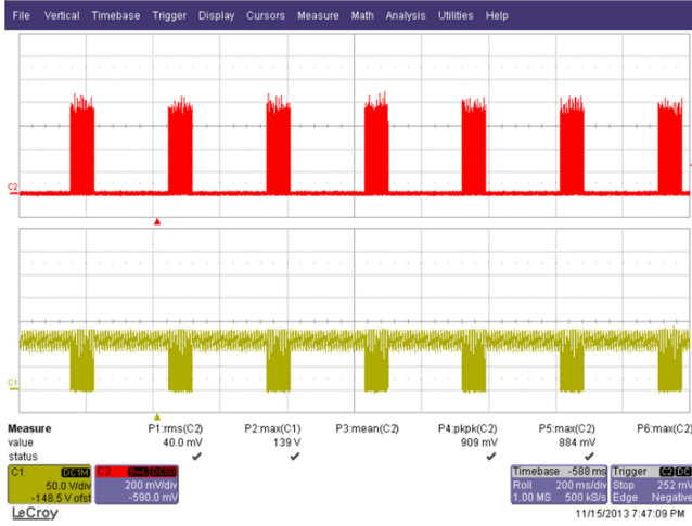
Figure 38 – 90 VAC, 60 Hz Output Short Condition. Upper: I_{DRAIN} , 500 mA / div. Lower: V_{DRAIN} , 100 V, 200 ms / div.
