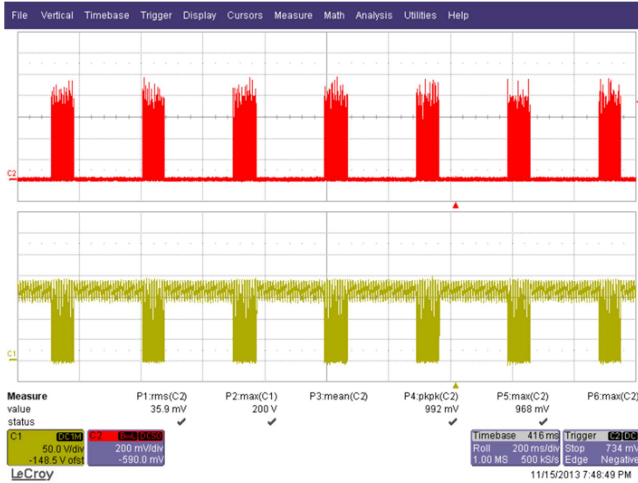
Figure 40 – 132 VAC, 60 Hz Output Short Condition. Upper: I_{DRAIN} , 500 mA / div. Lower: V_{DRAIN} , 100 V, 5 ms / div.
