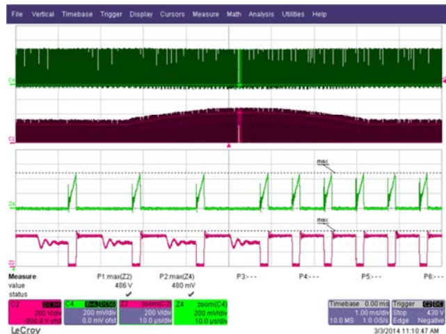
Figure 33 – 230 VAC, Full Load. Upper: I_{DRAIN} , 0.2 A / div. Lower: V_{DRAIN} , 200 V / div. Time Scale: 1 ms / div. Zoom Time Scale: 10 μs / div.
