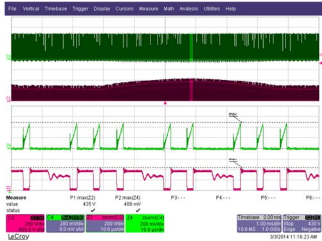
Figure 31 – 190 VAC, Full Load. Upper: I_{DRAIN} , 0.2 A / div. Lower: V_{DRAIN} , 200 V / div. Time Scale: 1 ms / div. Zoom Time Scale: 100 μs / div.
