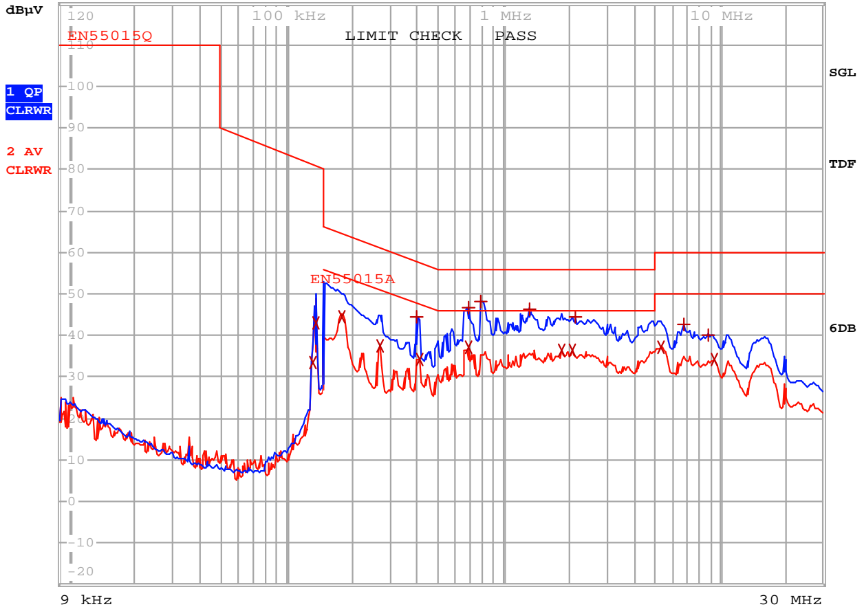
Figure 75 – Conducted EMI, Maximum Steady-State Load, 230 VAC, 60 Hz, and EN55015 B Limits. Unit on Top of Copper Plane that is Connected to Earth.
