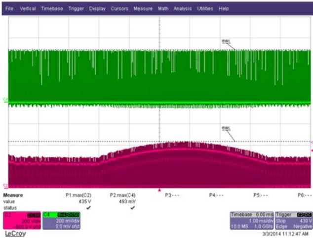
Figure 30 – 190 VAC, Full Load. Upper: I_{DRAIN} , 0.2 A / div. Lower: V_{DRAIN} , 200 V, 1 ms / div.
