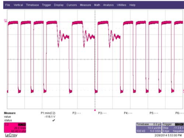
Figure 49 – 265 VAC Input and Full Load then Short. Upper: I_{DRAIN} , 0.2 A / div. Lower: V_{DRAIN} , 200 V / div. Time Scale: 50 μs / div. Zoom Time Scale: 2 μs / div.
