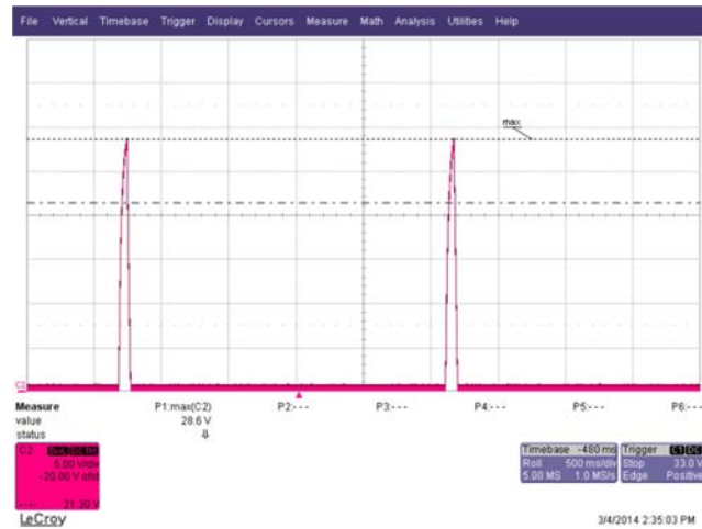
Figure 63 – 265 VAC Open Loop at Full-Load. V_{OUT} , 5 V / div. Time Scale: 500 ms / div.
