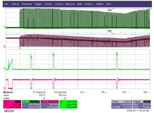
Figure 43 – 265 VAC Input and Shorted Load. Upper: I_{DRAIN} , 0.2 A / div. Lower: V_{DRAIN} , 200 V / div. Time Scale: 1 ms / div. Zoom Time Scale: 5 μs / div.
