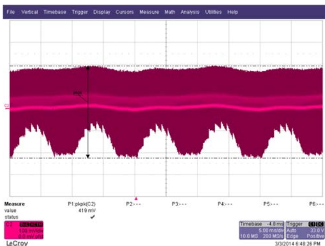
Figure 68 – Ripple, 230 VAC, Full Load. 5 ms, 100 mV / div.
