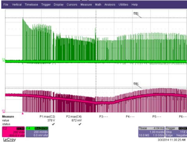
Figure 36 – 190 VAC Input and Maximum Load. Upper: I_{DRAIN} , 0.2 A / div. Lower: V_{DRAIN} , 200 V / div. Time Scale: 1 ms / div.
