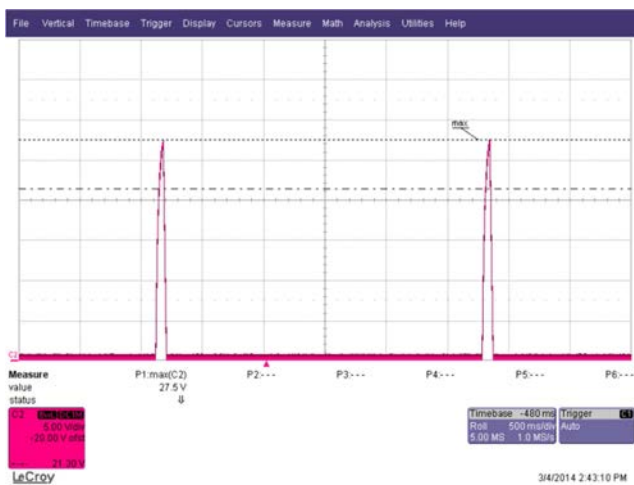
Figure 62 – 190 VAC Open Loop at Full-Load. V_{OUT} , 5 V / div. Time Scale: 500 ms / div.
