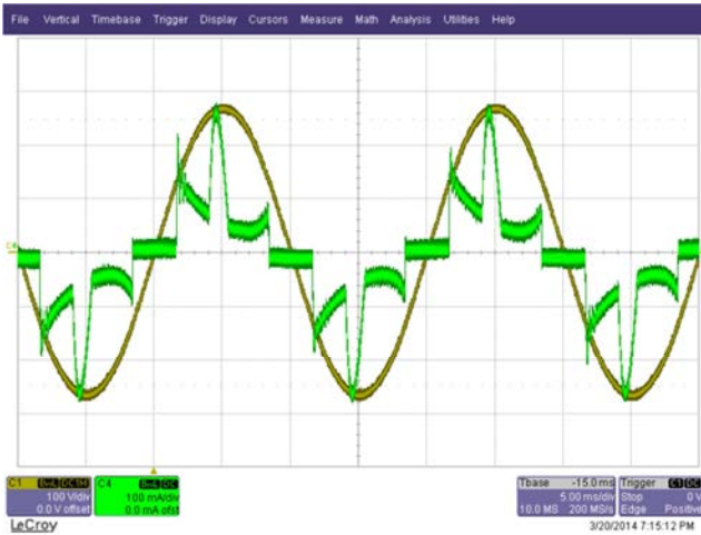
Figure 26 – 190 VAC, Full Load. Green: I_{IN} , 0.1 A / div. Yellow: V_{DIN} , 100 V, 5 ms / div.
