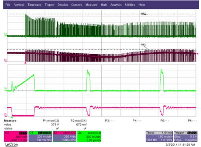
Figure 37 – 190 VAC Input and Maximum Load. Upper: I_{DRAIN} , 0.2 A / div. Lower: V_{DRAIN} , 200 V / div. Time Scale: 1 ms / div. Zoom Time Scale: 2 µs / div.
