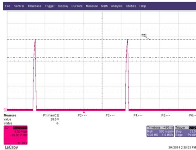
Figure 63 – 265 VAC Open Loop at Full-Load. V_{OUT} , 5 V / div. Time Scale: 500 ms / div.
