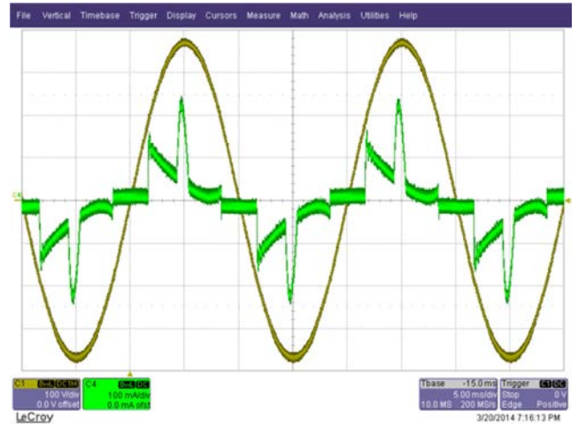
Figure 29 – 265 VAC, Full Load. Green: I_{IN} , 0.1 A / div. Yellow: V_{DIN} , 100 V, 5 ms / div.
