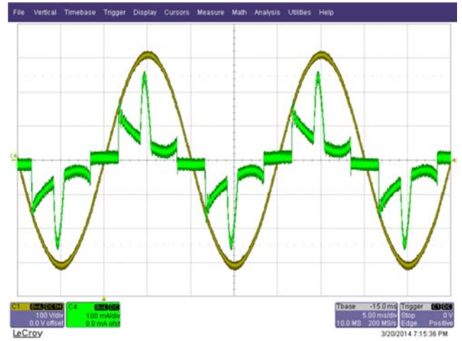
Figure 27 – 220 VAC, Full Load. Green: I_{IN} , 0.1 A / div. Yellow: V_{DIN} , 100 V, 5 ms / div.
