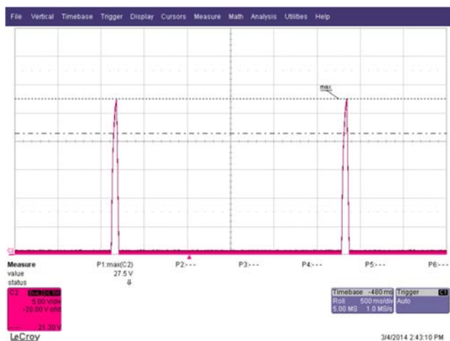
Figure 62 – 190 VAC Open Loop at Full-Load. V_{OUT} , 5 V / div. Time Scale: 500 ms / div.
