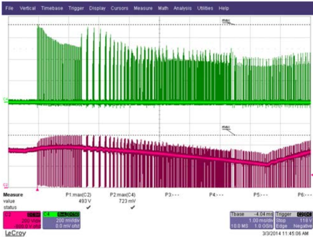
Figure 40 – 265 VAC Input and Maximum Load. Upper: I_{DRAIN} , 0.2 A / div. Lower: V_{DRAIN} , 200 V / div. Time Scale: 1 ms / div.
