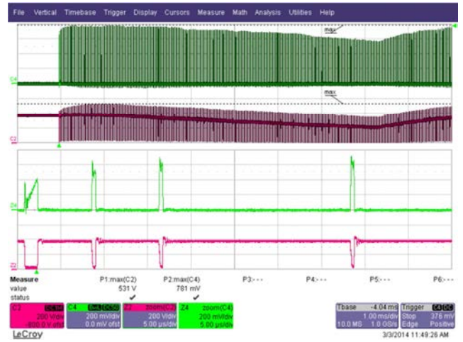
Figure 43 – 265 VAC Input and Shorted Load. Upper: I_{DRAIN} , 0.2 A / div. Lower: V_{DRAIN} , 200 V / div. Time Scale: 1 ms / div. Zoom Time Scale: 5 \mu s / div.
