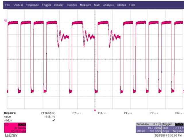
Figure 49 – 265 VAC Input and Full Load then Short. Upper: I_{DRAIN} , 0.2 A / div. Lower: V_{DRAIN} , 200 V / div. Time Scale: 50 \mu s / div. Zoom Time Scale: 2 \mu s / div.
