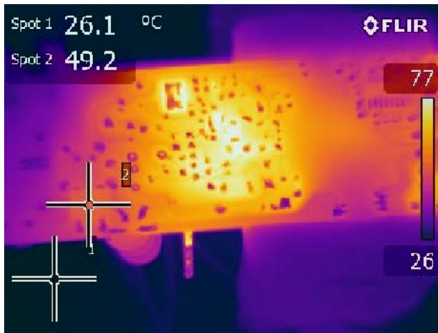
Figure 29 – 300 V VAC, Full Load. Spot 2: Bridge Diode (BR1): 49.2 °C.
