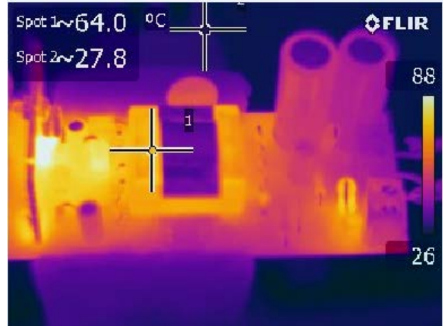
Figure 26 – 300 V VAC, Full Load. Spot 1: Transformer (T1): 64 °C.
