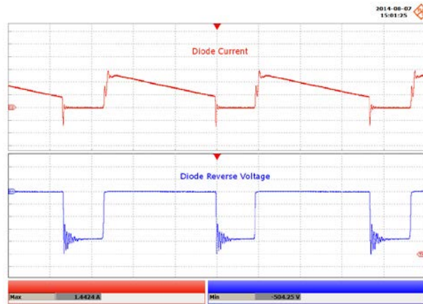
Figure 83 – 265 VAC, 95 V LED Load, Normal. Upper: I_{DIODE} , 500 mA / div. Lower: V_{DIODE} , 100 V / div., 2 \mu s / div. Peak I_{DIODE} : 1.442 A. Peak Diode Reverse Voltage: 504.25 V.
