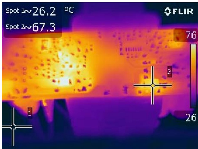
Figure 39 – 170 V VAC, Full Load. Spot 2: Output Diode (D16): 67.3 °C.
