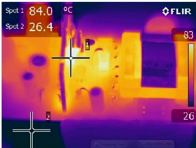
Figure 37 – 170 V VAC, Full Load. Spot 1: LYT4325E (U1): 84 °C.
