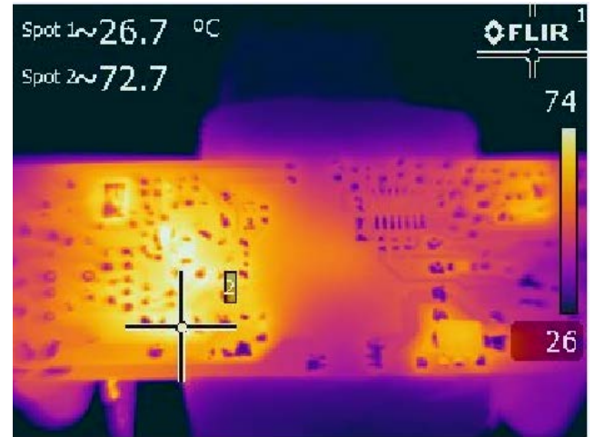
Figure 34 – 230 V VAC, Full Load. Spot 2: Blocking Diode (D7): 72.7 °C.
