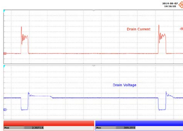
Figure 75 – 170 VAC, 95 V LED Load, Start-up. Upper: I_{DRAIN} , 400 mA / div. Lower: V_{DRAIN} , 100 V / div., 2 μs / div. Peak I_{DRAIN} : 2.307 A. Peak V_{DRAIN} : 389.19 V.
