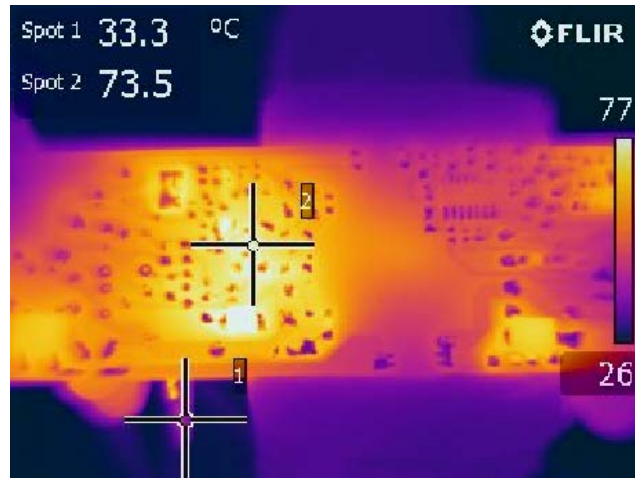
Figure 41 – 170 V VAC, Full Load. Spot 2: Blocking Diode (D8): 73.5 °C.
