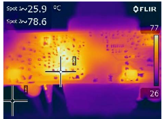
Figure 40 – 170 V VAC, Full Load. Spot 2: Blocking Diode (D7): 78.6 °C.
