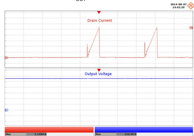
Figure 87 – 170 VAC, No LED Load. Upper: I_{DRAIN} , 200 mA / div. Lower: V_{OUT} , 20 V / div., 4 \mu s / div. Peak I_{DRAIN} : 1.166 A. Peak V_{OUT} : 113.18 V.
