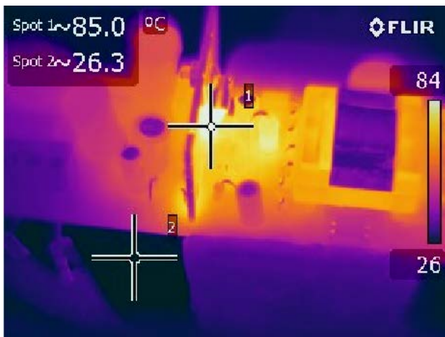
Figure 31 – 230 V VAC, Full Load. Spot 1: LYT4325E (U1): 85 °C.
