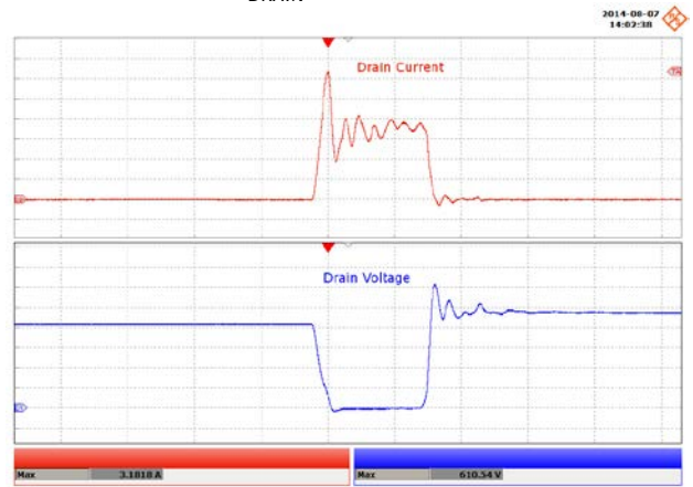
Figure 81 – 300 VAC, Output Short. Upper: I_{DRAIN} , 500 mA / div. Lower: V_{DRAIN} , 100 V / div., 400 ns / div. Peak I_{DRAIN} : 3.182 A. Peak V_{DRAIN} : 610.54 V.
