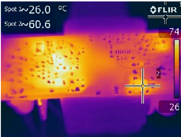
Figure 33 – 230 V VAC, Full Load. Spot 2: Output Diode (D16): 60.6 °C.
