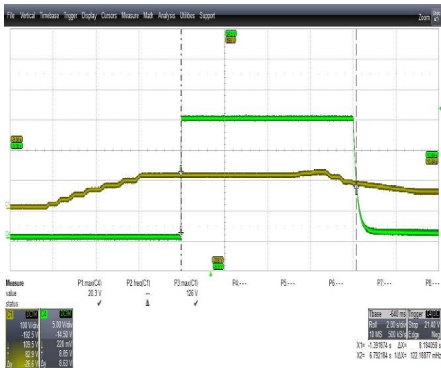
Figure 52 – Line Undervoltage. DC Input, No-Load. V_{UV+} : 109.5 V, V_{UV-} : 82.9 V. Upper: Input, 100 V. Lower: V_{OUT} , 5 V, 2 s / div.
