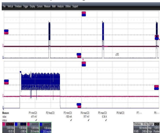
Figure 38 – Output Voltage and Current Waveforms. 90 VAC Input. Upper: V OUT , 5 V. Lower: I OUT , 1 A, 0.5 s, 20 ms / div.
