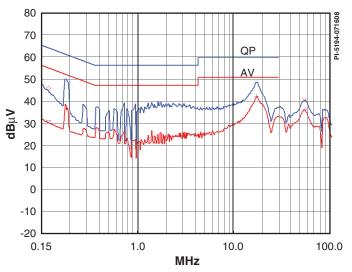
Figure 3. Conducted EMI Scan, EN55022 B Limits. Measurements Made at 230 VAC with Output RTN Grounded.
