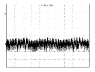
**Figure 23** – Ripple, 115 VAC, Full Load. 5 ms, 50 mV / div (80 mV<sub>P-P</sub>).
