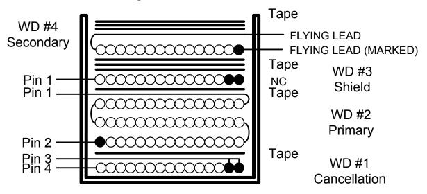
Figure 6 – Transformer Build Diagram.
