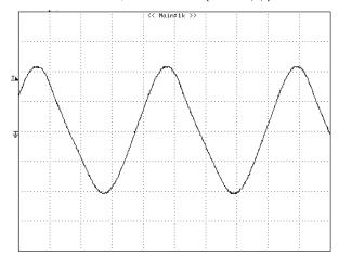
Figure 25 – Ripple of a Linear adaptor, 115 VAC Input, Full Load.
