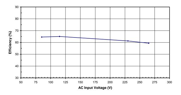
Figure 7 - Efficiency vs. Input Voltage, Room Temperature, 60 Hz.
