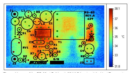
Figure 11 – Thermal Image of the RD-83 at Full Load, 85 VAC Input and Ambient Temperature of 22 °C.
