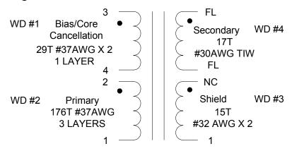
Figure 5 - Transformer Electrical Diagram.
