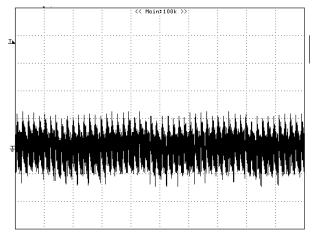
**Figure 24** – Ripple, 230 VAC, Full Load. 5 ms, 50 mV /div (130mV<sub>P-P</sub>).
