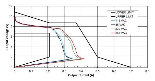
Figure 10 – Output VI Curve, Room Temperature.
