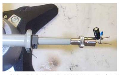
Figure 21 – Oscilloscope Probe with Probe Master 5125BA BNC Adapter (Modified with wires for probe ground for ripple measurement, and two parallel decoupling capacitors added).
