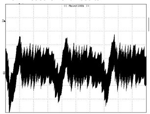
Figure 22 – Ripple, 85 VAC, Full Load. 5 ms, 50 mV / div (240 mV<sub>P-P</sub>).
