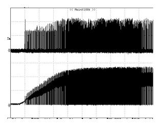
Figure 17 – 265 VAC Input and Maximum Load. Upper: I<sub>DRAIN</sub>, 0.1 A / div. Lower: V<sub>DRAIN</sub>, 200 V & 1 ms / div.
