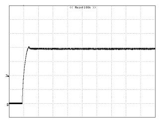
Figure 14 – Start-up Profile, 115VAC. 2 V, 20 ms / div.
