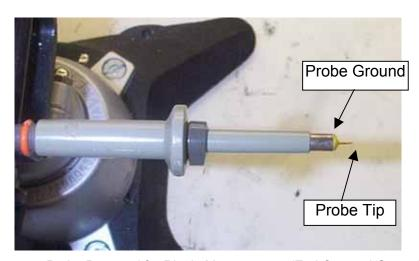
Figure 20 - Oscilloscope Probe Prepared for Ripple Measurement (End Cap and Ground Lead Removed).
