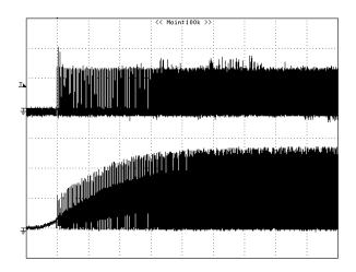
Figure 16 – 85 VAC Input and Maximum Load. Upper: I<sub>DRAIN</sub>, 0.1 A / div. Lower: V<sub>DRAIN</sub>, 100 V & 1 ms / div.
