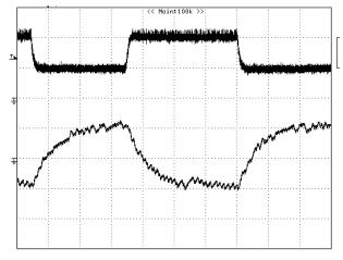
Figure 18 – Transient Response, 115 VAC, 50-100-50% Load Step.
