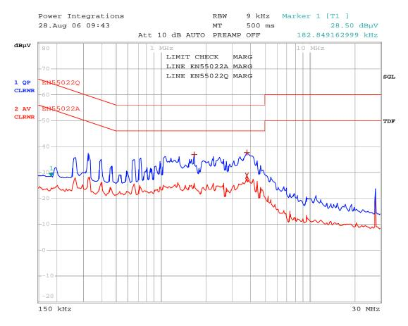
Figure 26 - Conducted EMI, Maximum Steady State Load, 115 VAC, 60 Hz, and EN55022 B Limits.
